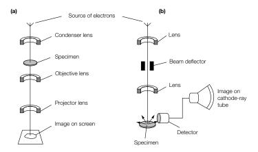
Fig. 4. Principal features of (a) a transmission electron microscope and (b) a scanning electron microscope.
